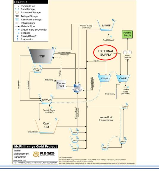
The project's water management system is designed to provide sufficient capacity in the mine water management storages to avoid discharges during periods of high rainfall ...
