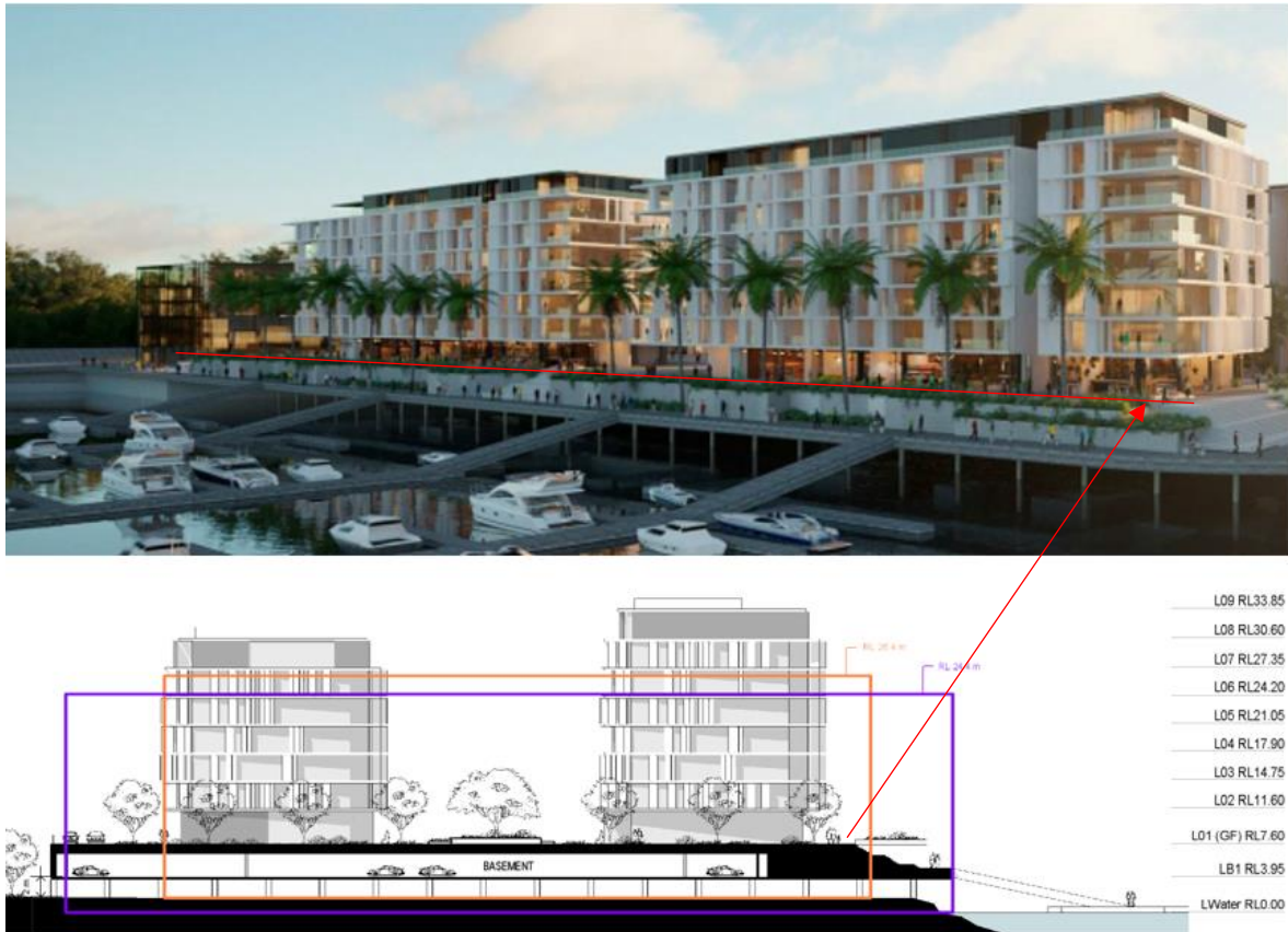
Figure 7: The planning proposal building design is shown above, where the building platform is at 7.6m below that is only basement and piers.
