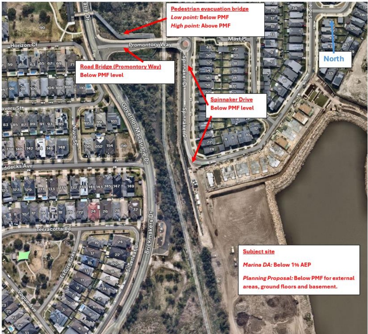
Figure One: Moorebank East precinct indicating levels of structures compared to flood levels.
