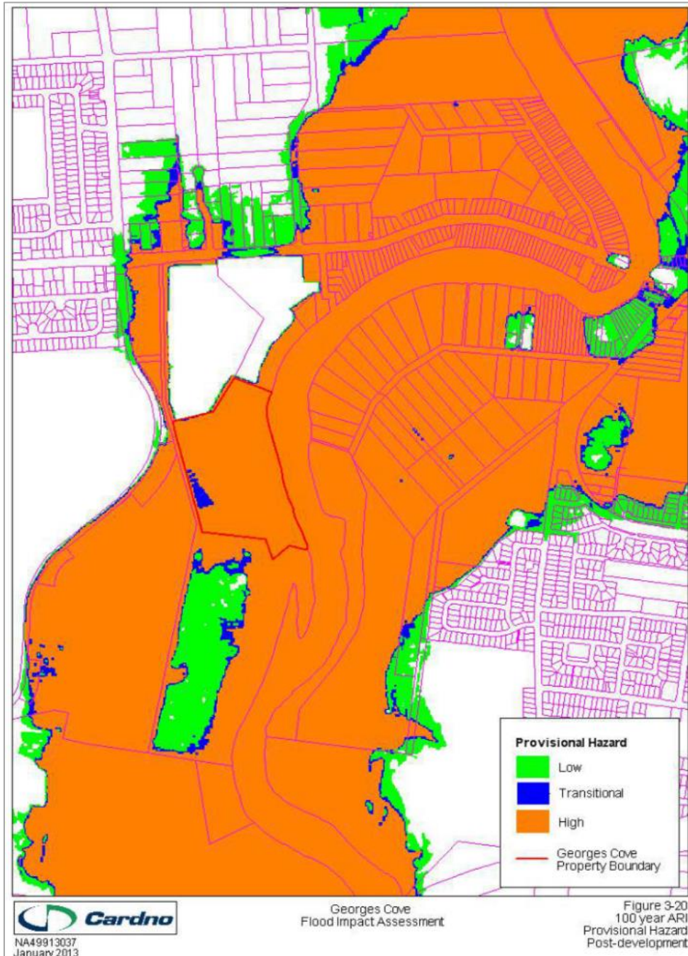
Figure Two: Flood Impact Assessment for the proposed Georges Cove Marina, Moorebank; dated: 29 January 2013, Cardno
