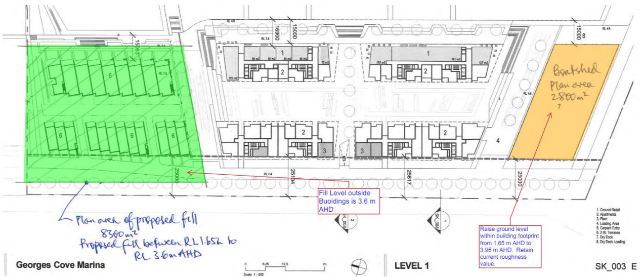
Figure 5 Excerpt of Flood Impact Assessment – Concept plan showing filling modifications to facilitate development envisaged in the planning proposal
