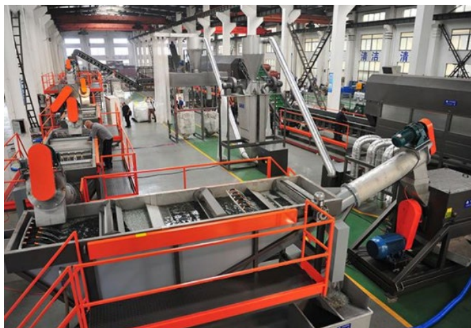
Figure 10 | Example of PET bottle washing and recycling lines
