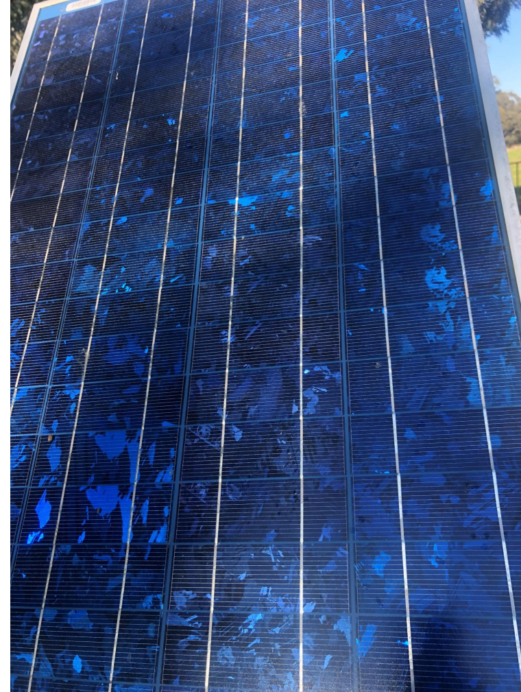
Solar panel breaking down after 10 years
