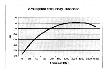
This A scale weighting is the most popular standard and it is used because it records and model the production and perception of the human voice. The curve shows omission of LFN.
