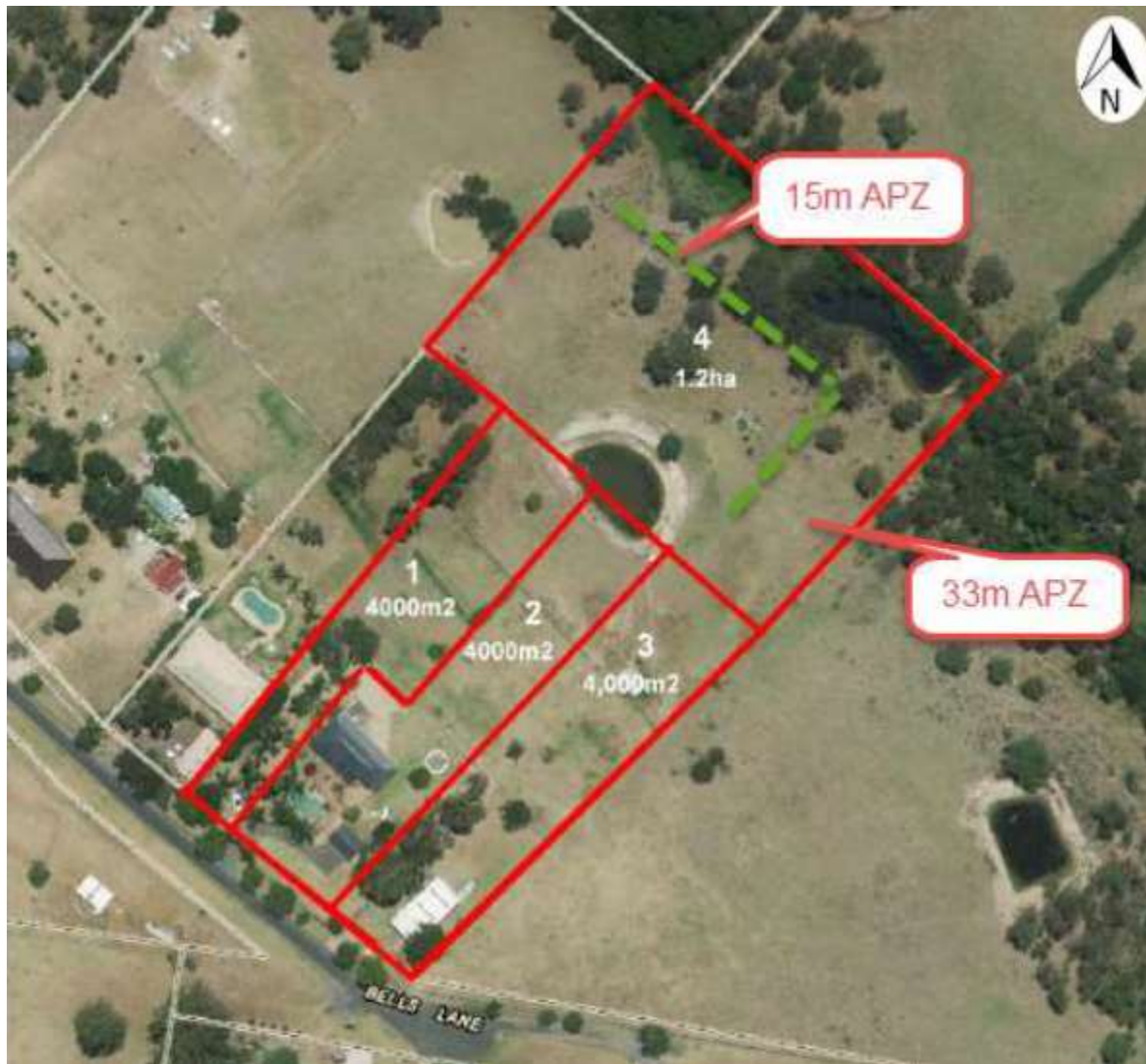
Image 7 – Indicates the APZs for the Classified Vegetation to the North and East of the proposal (Montgomery Planning Solutions 2019), The APZ to the North is from the vegetation on the banks of the creek line.
