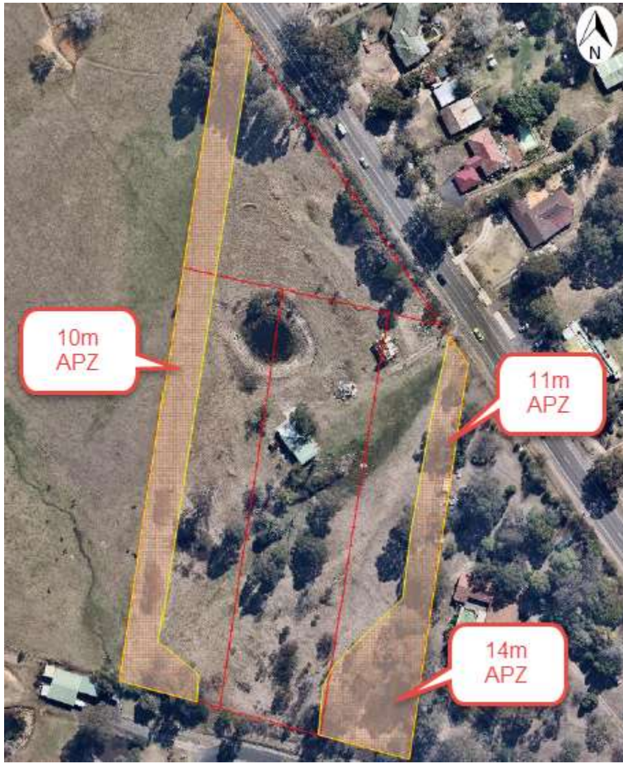
Image 12 – Indicates the potential locations for a building envelope regarding the vegetation type and slope to ensure that the BAL does not exceed BAL 29. The APZ required for the Grassland Classified Vegetation to the West is 10m minimum; the APZ required for the South is 14m minimum and; the APZ for the East 11m minimum. There is sufficient room on the proposed allotments for a dwelling and necessary APZ areas.
