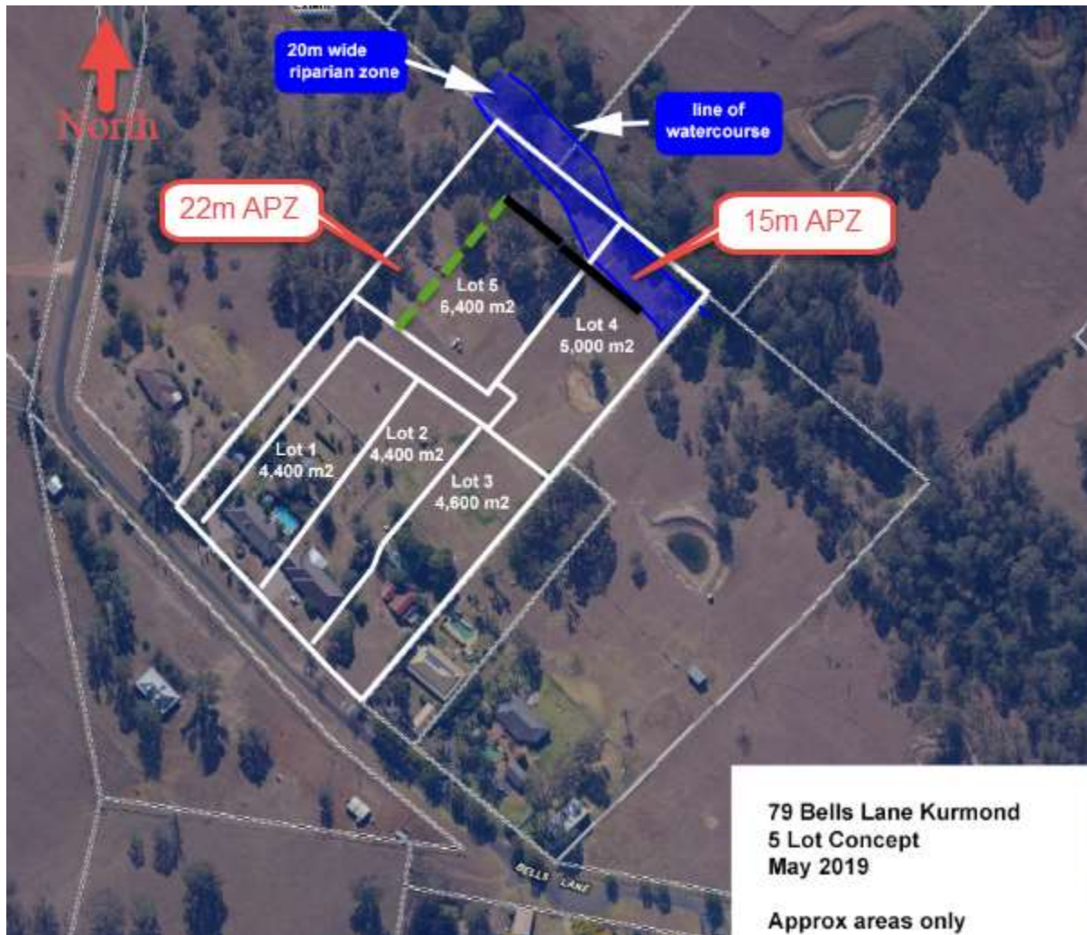
Image 4 – Indicates the 22m APZ required for the Western boundary and 15m Northern boundary of Lot 5 and the Northern and Eastern boundary of Lot 4 for compliance with PBP 2006 and AS3959-2009 (note the APZs in this image is for BAL-29 Construction).
