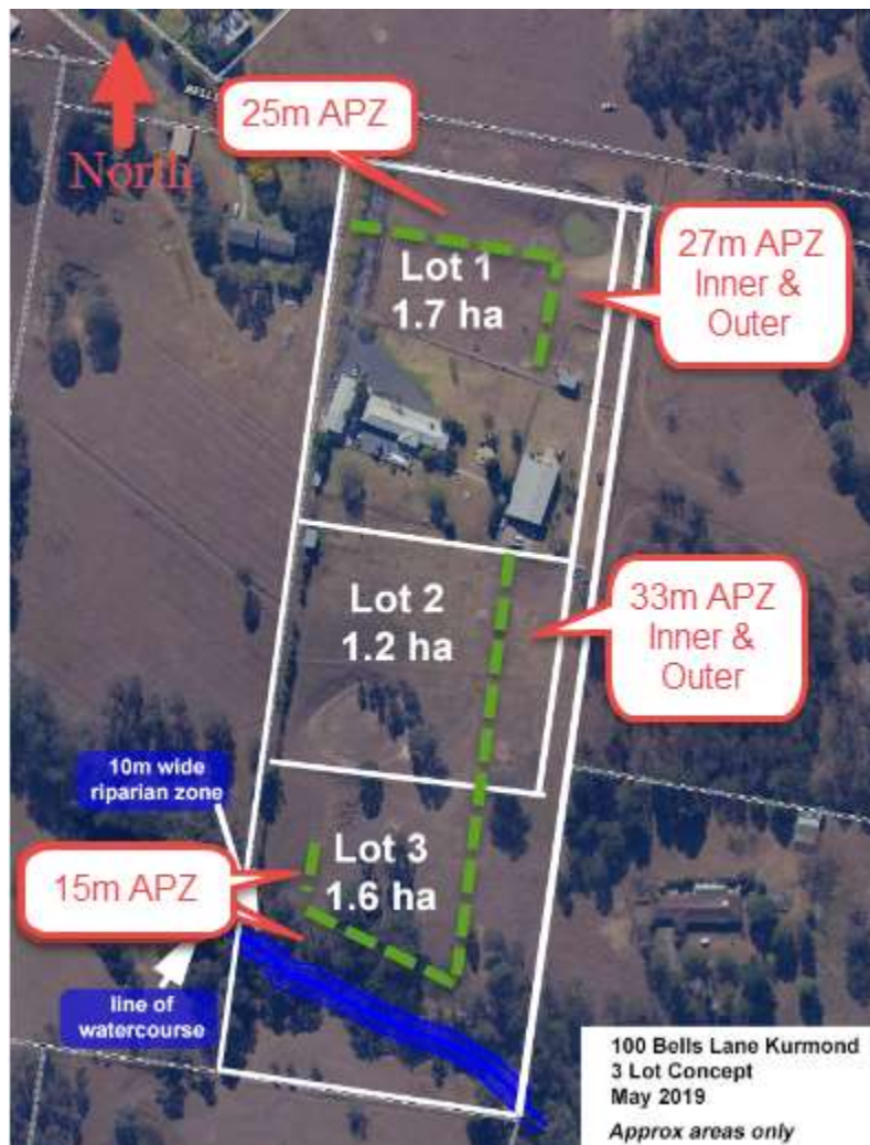
Image 10 - Indicates the min APZs required for compliance with PBP 2006 and AS3959-2009. Note APZs are located only on the subject Lot and not in neighbouring properties. Note the APZs in this image is for BAL-29 Contrsuction.
