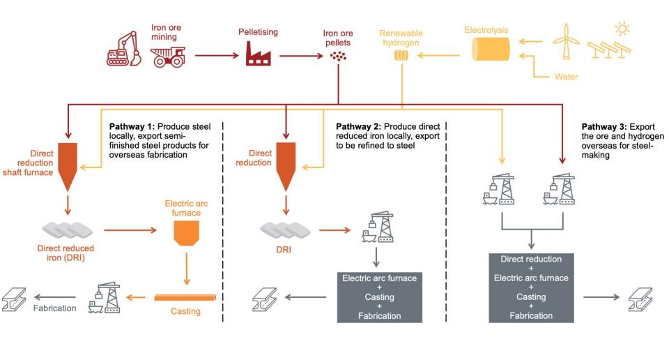
Notes: All three pathways require low-emissions electricity in each step. Iron ore mining and pelletising need not occur in Australia.
