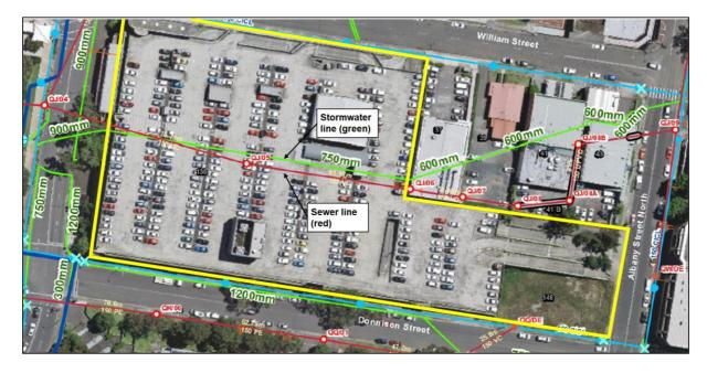
Figure 26 | Location of stormwater (green) and sewer (red) pipes crossing the site (yellow) (Base source: Applicant's EIS)
