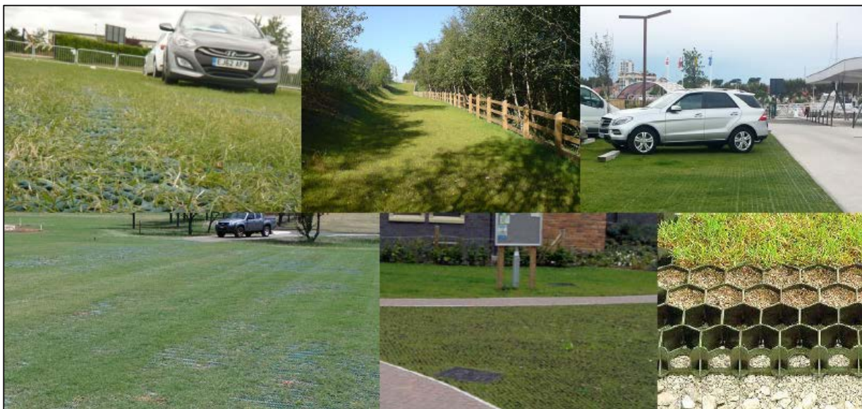
Picture 14 – Examples of reinforced grass parking areas
