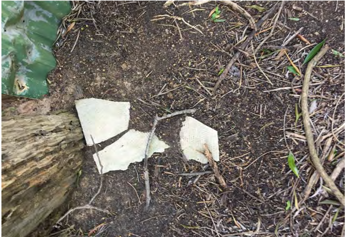
Photo 5 - Fragments of bonded ACM visible at TP39
