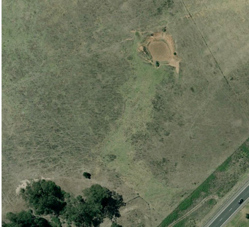
Photo 32 – Drainage line 1, site inspection revealed a grass swale below a small breached Dam 12 with no defined channel
