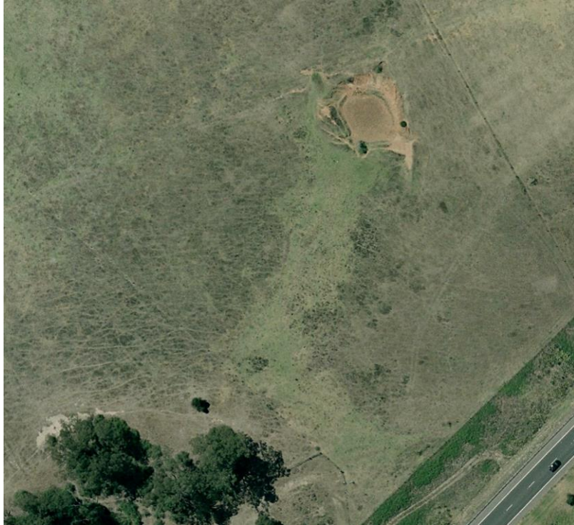
Photo 32 – Drainage line 1, site inspection revealed a grass swale below a small breached Dam 12 with no defined channel on the adjoining Lot (offsite)
