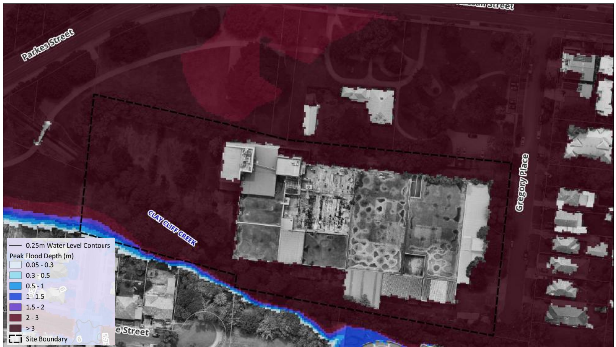
Figure 29 | Pre-development PMF riverine flood depth (Source: Rhelm)
