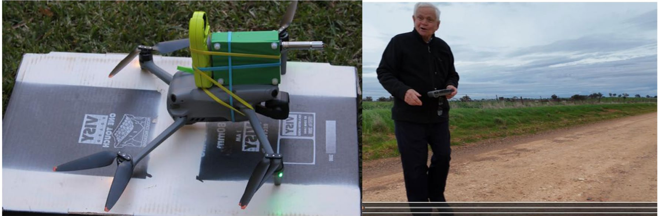
Figure 7a. Air2 showing mounting of green Vaisala-tracker with lime Kestrel 520 Meter.
