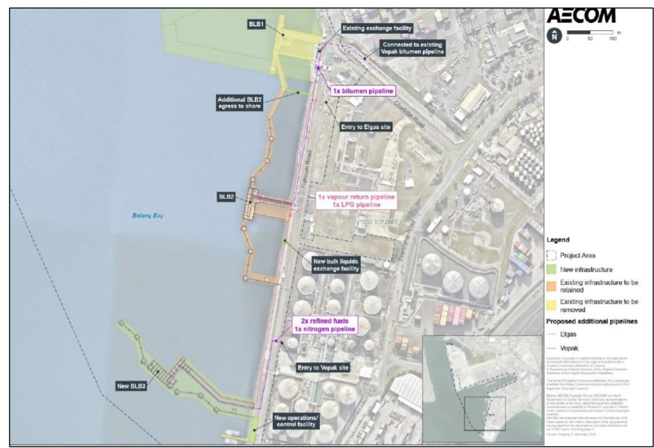
Figure 14 | Bulk liquids berths and pipelines at Port Botany (Source: EIS, Appendix G)
