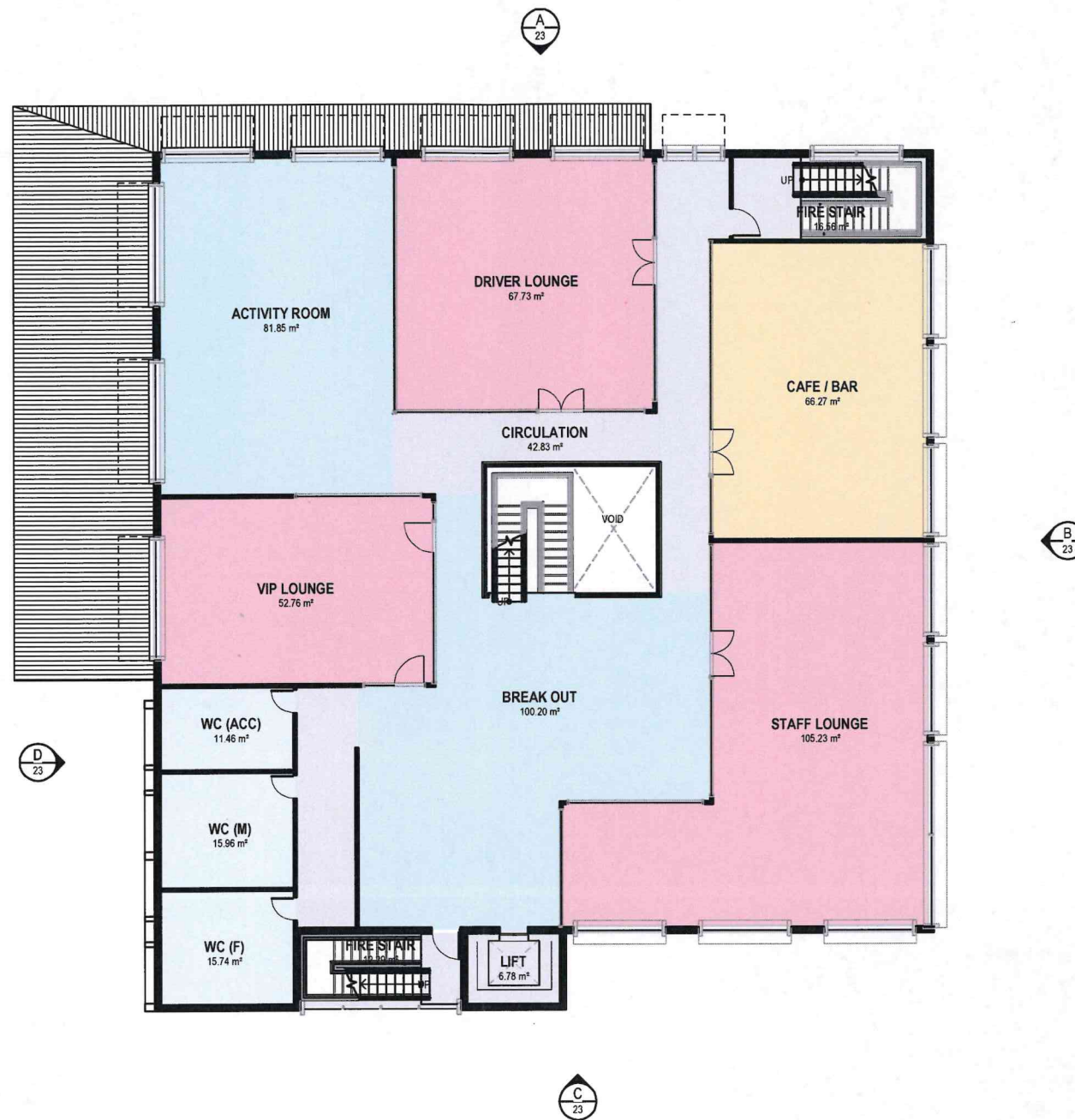
ADMIN BUILDING - LEVEL 1 FLOOR PLAN
