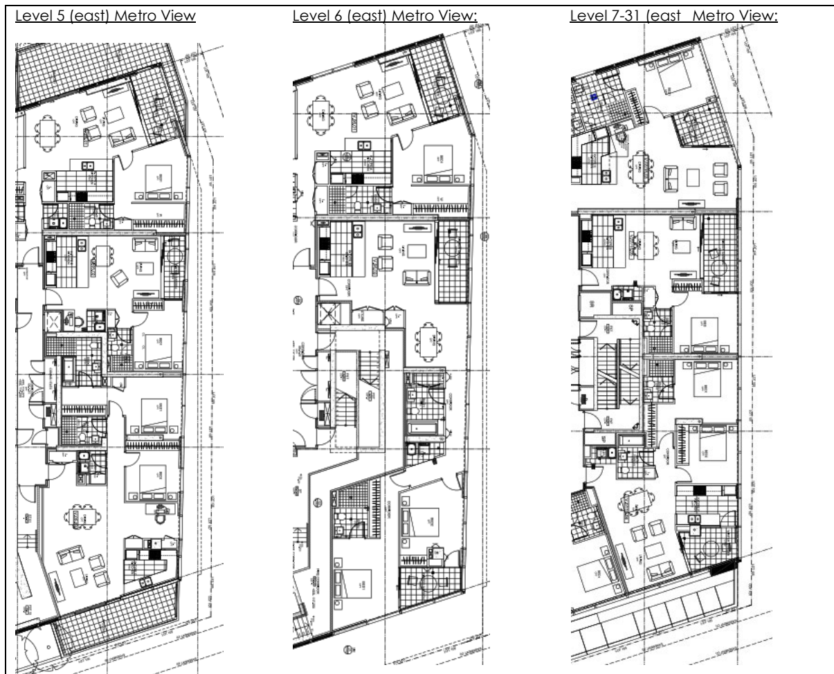
Figure 4: Extracts from 'As Built' Plans of Metro View showing units layout in eastern side of Levels 5-31 (Source: client)
