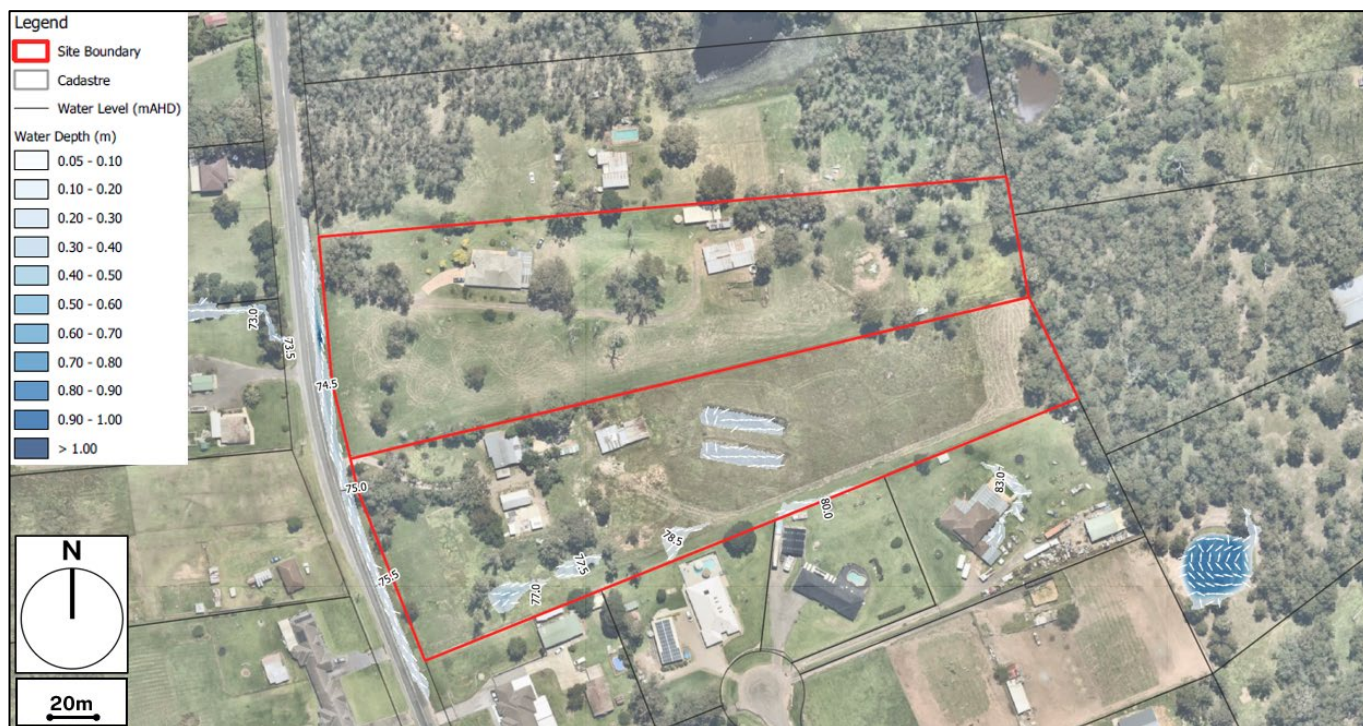
Figure 11 | Existing 1% AEP flood water level and depth (Source: Applicant's response to Further Request for Information (RFI), 2025)
