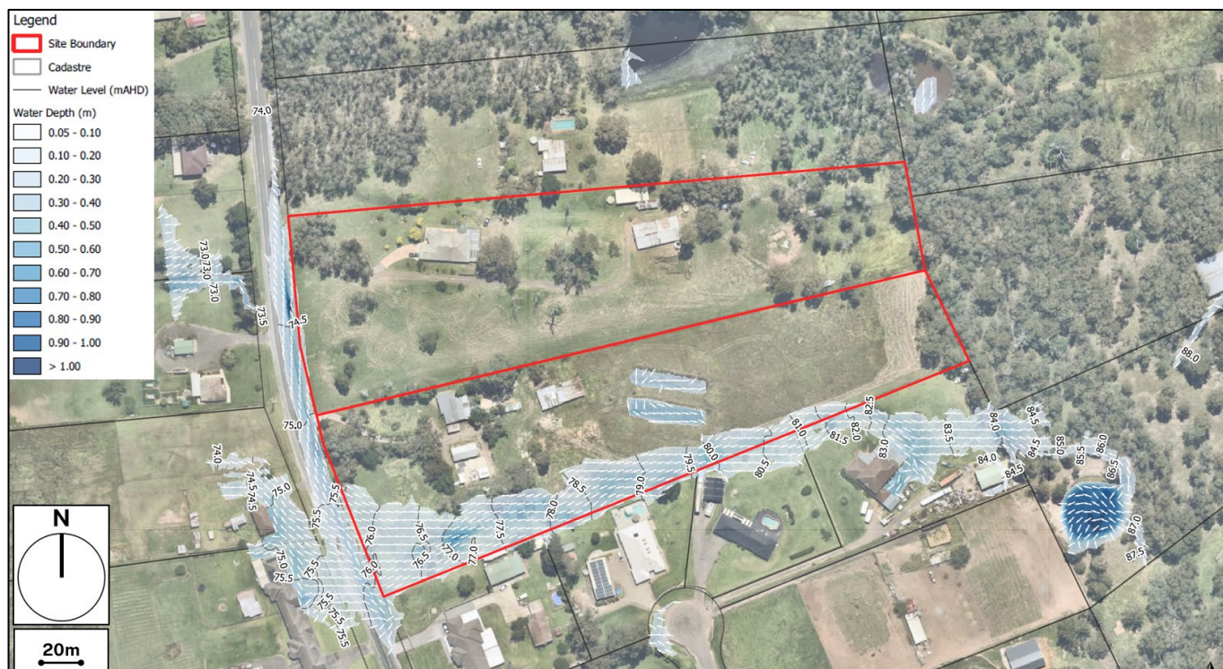
Figure 12 | Existing PMF flood water level and depth (Source: Applicant's response to Further RFI, 2025)
