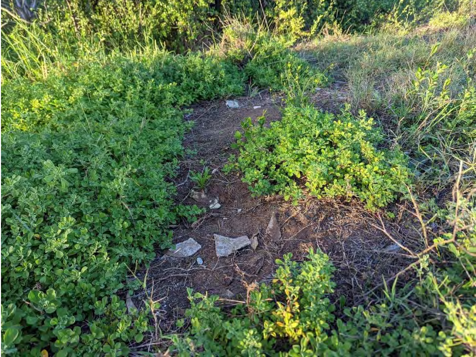
Photo 3: Location 14 – Visible and accessible ACM debris identified on the site surface prior to removal work
