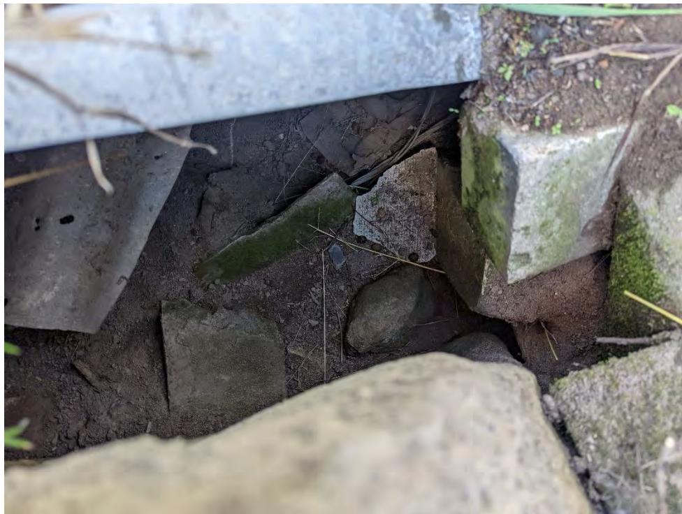
Photo 22: Location 25 – Cement sheeting visible within rubbish dump prior to asbestos removal work
