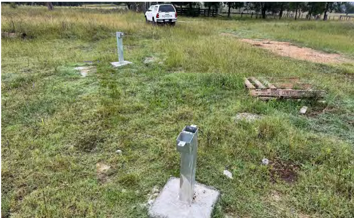
Photo 4: Newly installed groundwater monitoring wells (TL3) near cattle yards, looking east.
