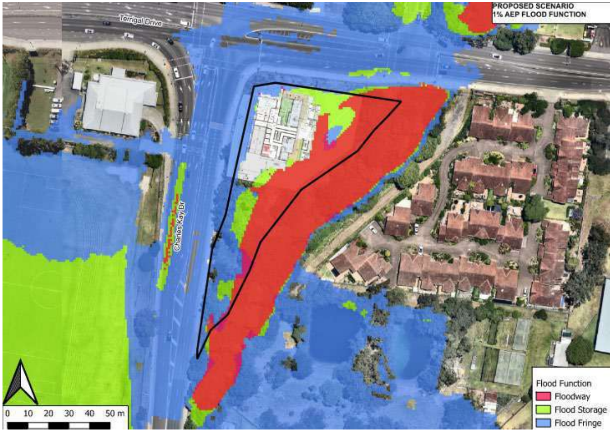
Figure 12 - 1%AEP_Post Development Flood Function
