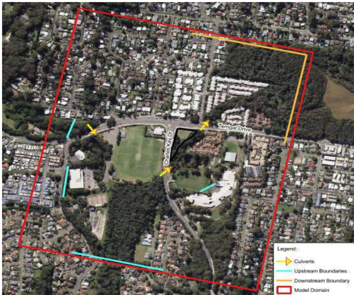
Figure8 - Grid & Boundary Condition Details
