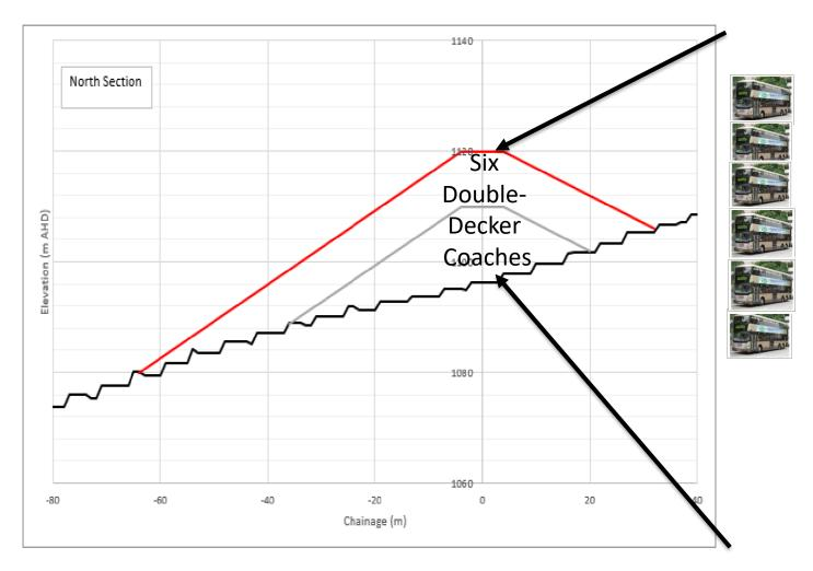
Inset 10: Schematic cross sections through the TT embankment where it crosses the deeply incised drainage paths
