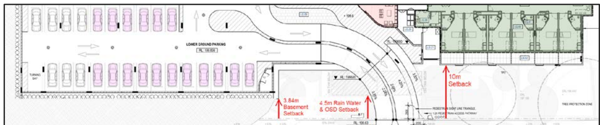
Figure 15 | Part lower ground floor plan showing the basement and OSD encroachment into the front setback (Base Image Source: Architectural Plans)
