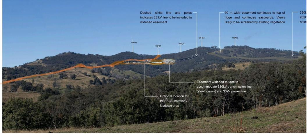
**Figure B.1.1.2**. Transmission Line (Option 1) Photomontage PM01 (Representative of AD\_74) Note: The photomontage demonstrates location and course of power lines for representation purposes only. The proposed power lines will be of subtle colour and will blend w
