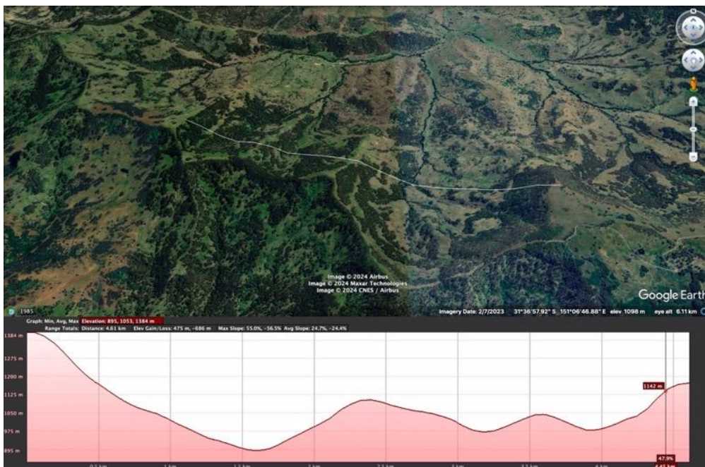
Figure 4 Google earth oblique straight line cross section between towers 13 and 20. Maximum slope is 56.5 percent and average slope around 24.5 percent. Location of the cross section is also shown in figure 5
