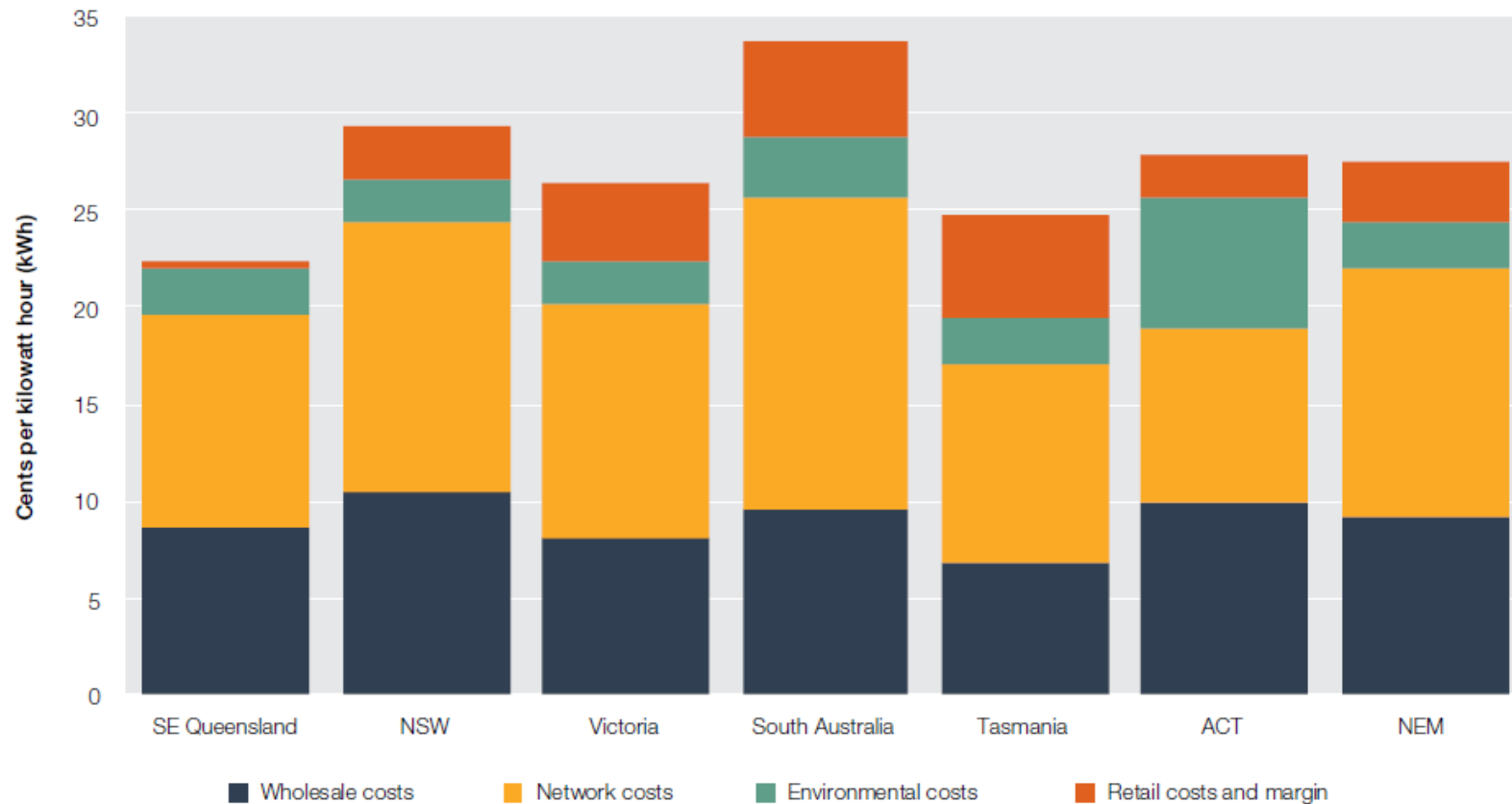
Figure 6.2 Composition of a residential bill – electricity
