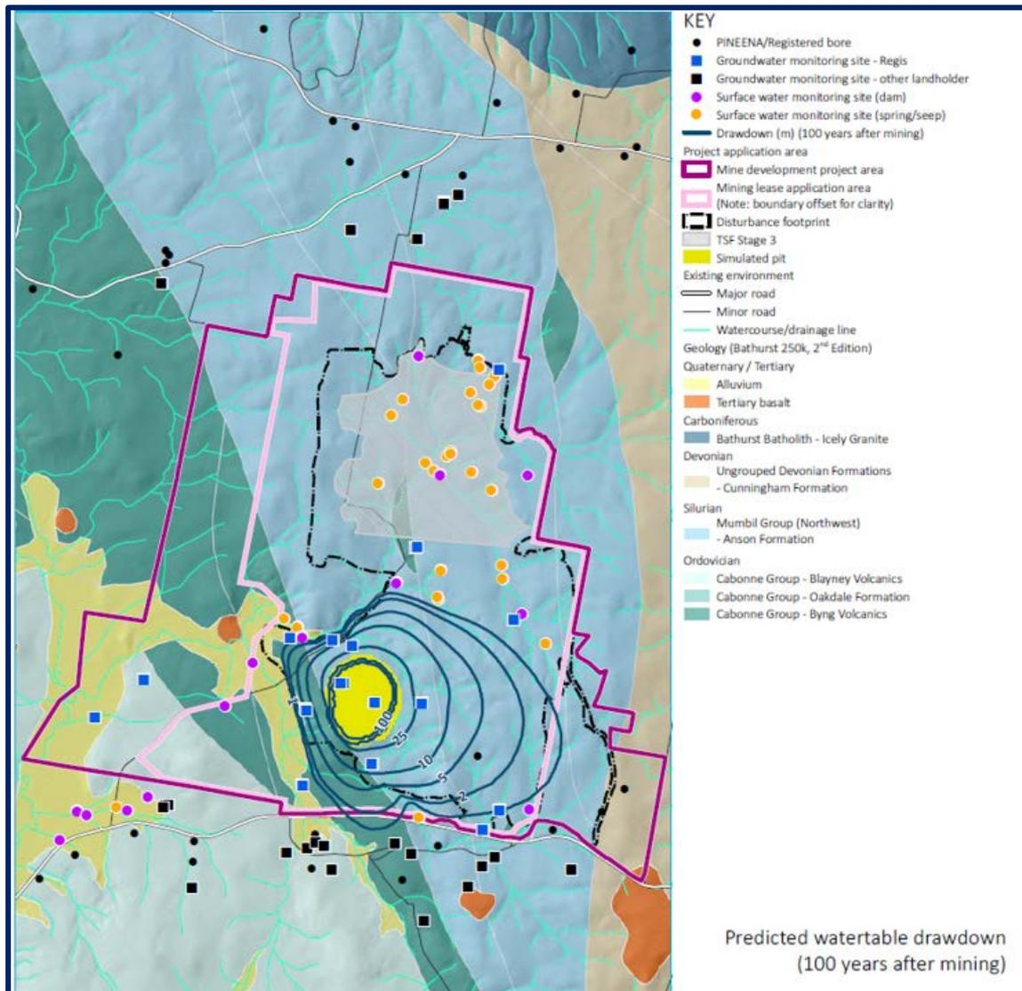
**Figure 14 |** Predicted groundwater drawdown – 100 years post-mining (Source: First Amendment Report, Appendix H (September 2020))
