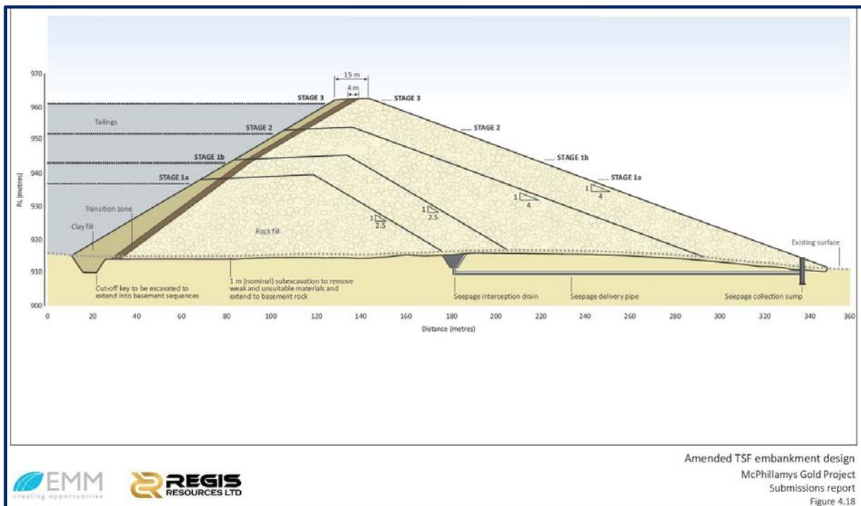
**Figure 12:** Mine TSF Embankment design and construction (Source: Submissions Report (September 2020))
