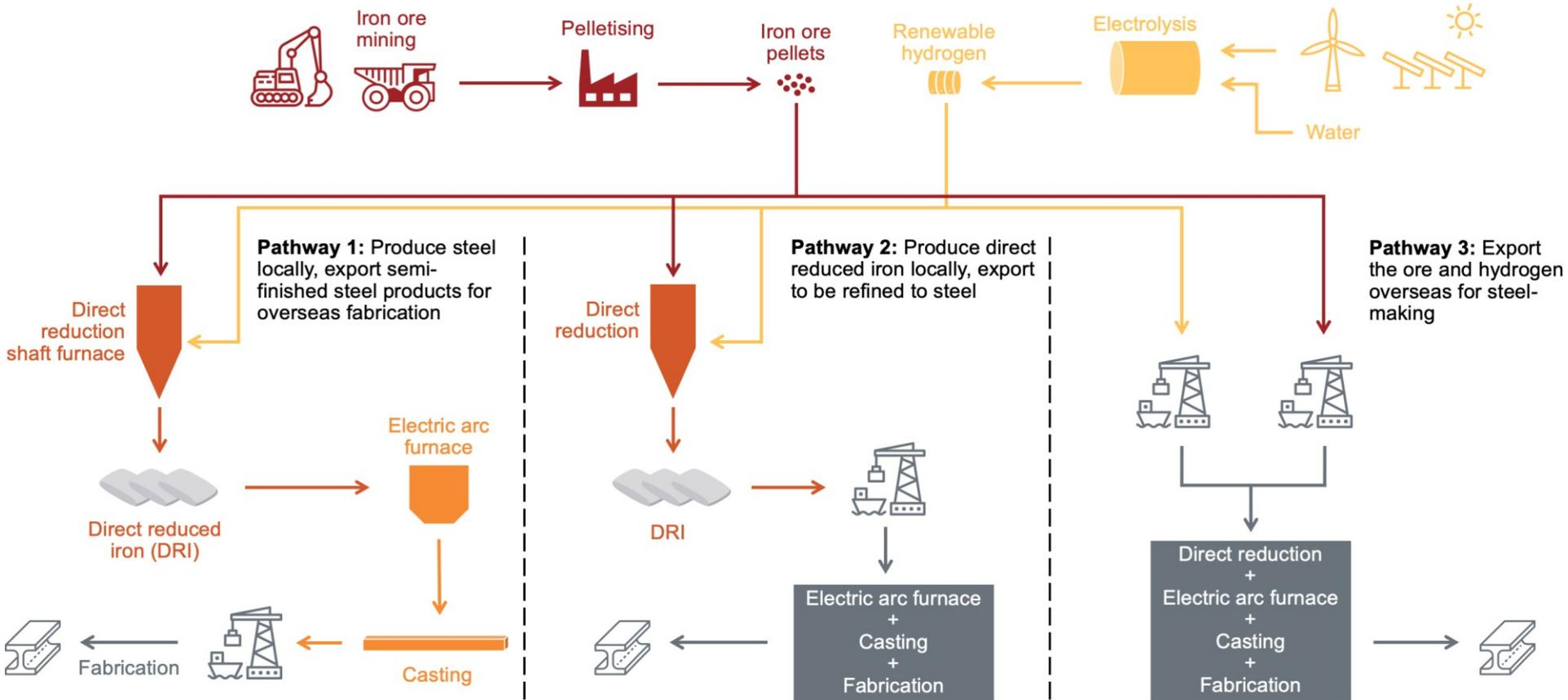
Notes: All three pathways require low-emissions electricity in each step. Iron ore mining and pelletising need not occur in Australia.
