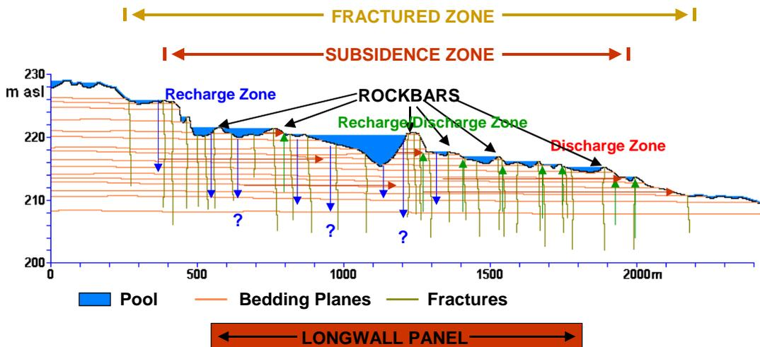
Figure 4. Simplified concept of longitudinal SW-GW interaction in a longwall mining impacted catchment.
