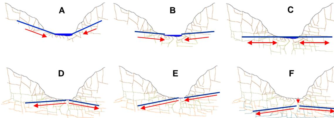
Figure 3. Conceptual model of various scenarios of SW-GW interaction in a longwall mining impacted catchment. Time scale scenarios from natural system (A) to possible final impacted system (F).
