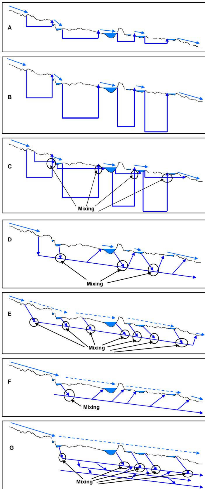
Figure 5. Possible scenarios of SW-GW interaction along a river depending on the level of subsidence-induced fracturing and bedding plane distribution.
