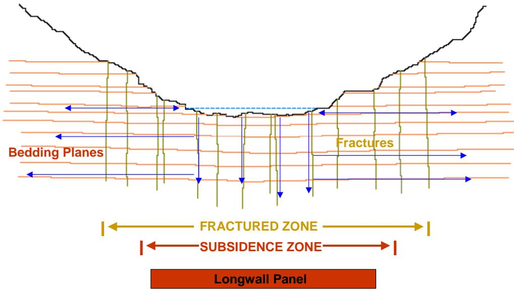
Figure 2. Concept of lateral SW-GW interaction in a longwall mining impacted catchment.
