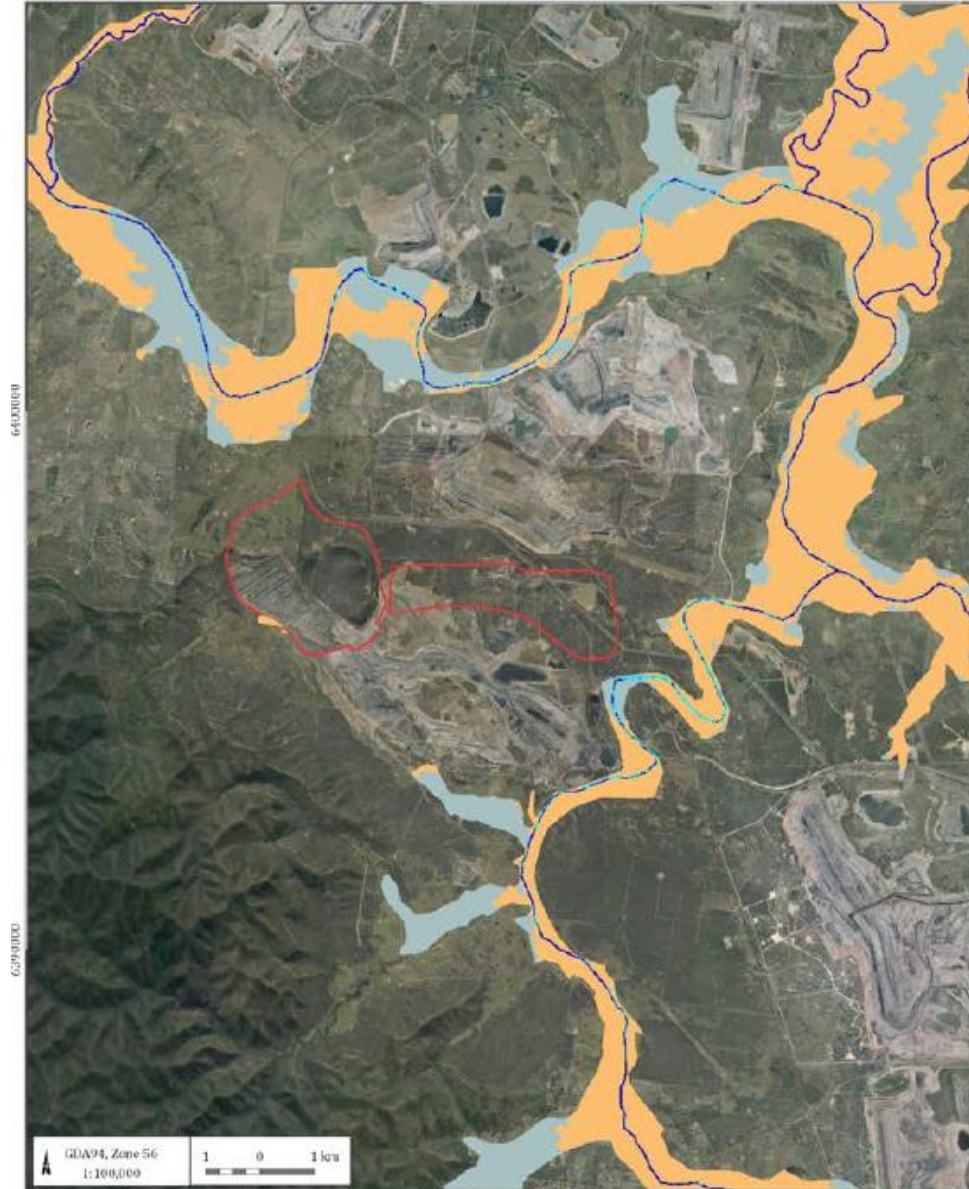
United Wambo Project - Groundwater Impact Assessment (G1733) Interpolated gaining and losing stream and alluvial zones
