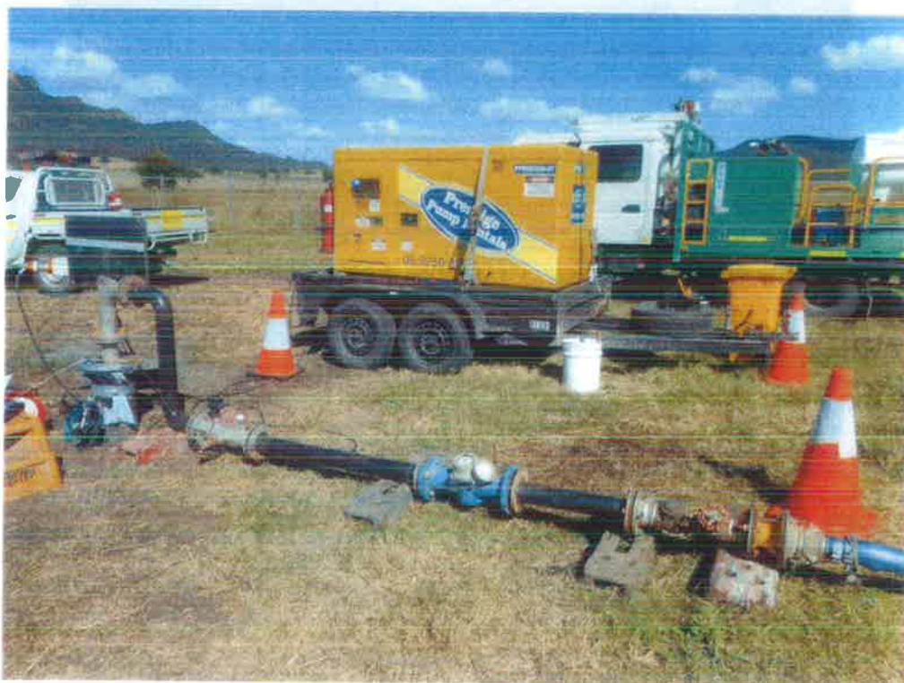
Figure 4-10 Headworks and flow meter setup
