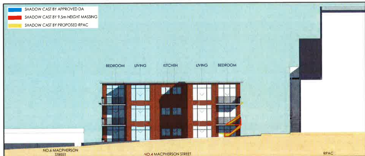
Figure 39: RPAC shadow on northern elevation of 4 Macpherson St during mid-winter at 2pm
