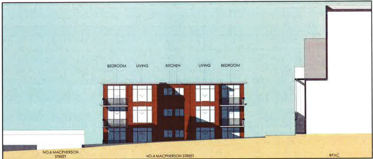
Figure 37: Sunlight to the northern elevation of 4 Macpherson St during mid-winter at 9am
