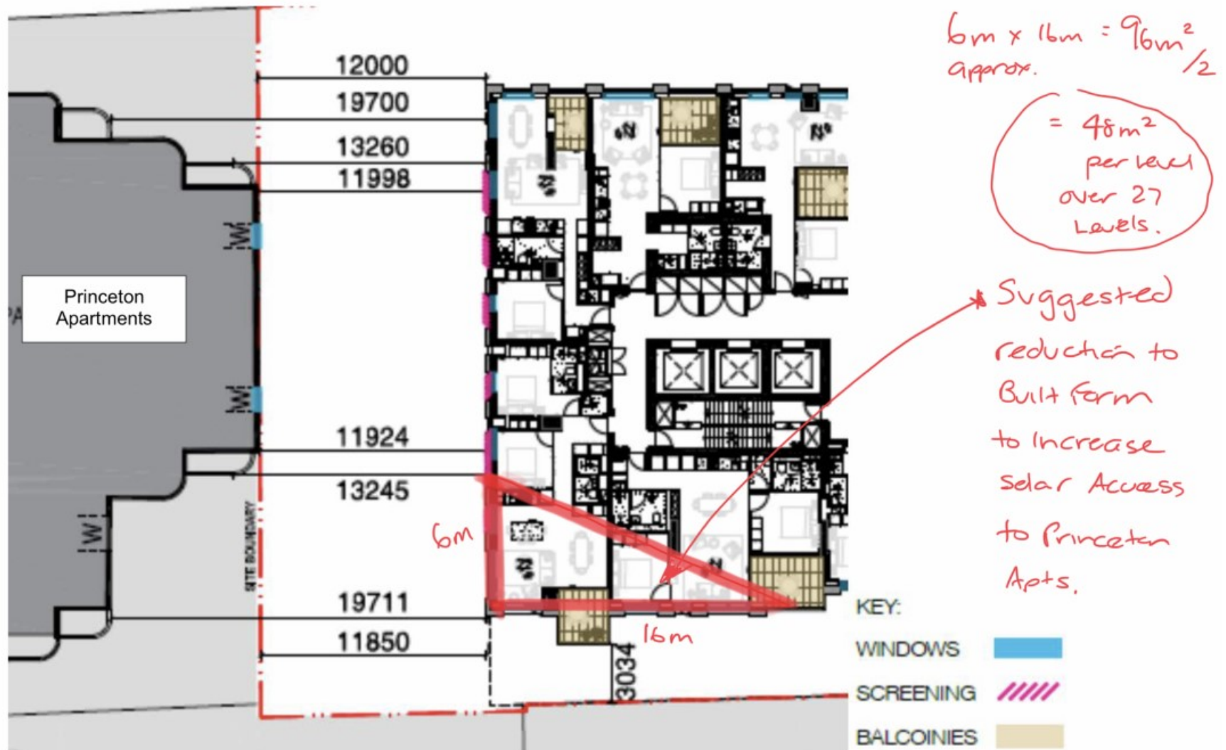
Figure 25 | Building separation distances (in mm) between proposed building and Princeton Apartments (Base source: RTS)
