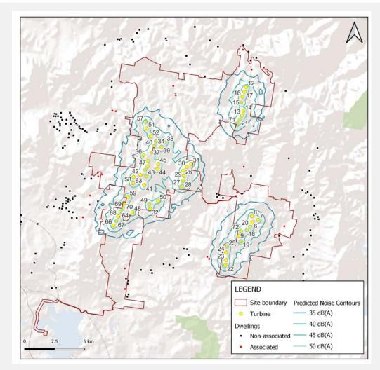
Figure: Predicted operational noise levels.
