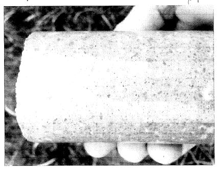
Photograph 1: DCQ rhyolite from diamond drill core
