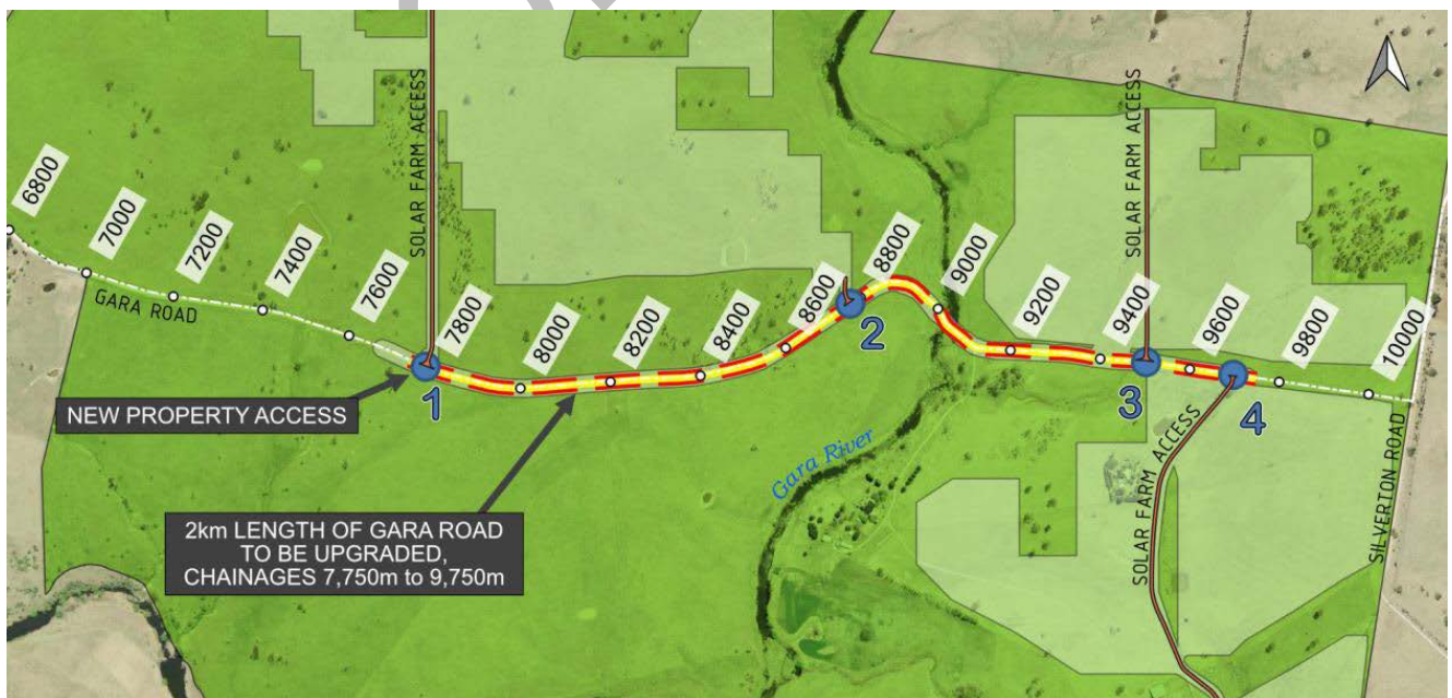
Figure 1 Gara Road Upgrade extent and Secondary Access Points 1 to 4
