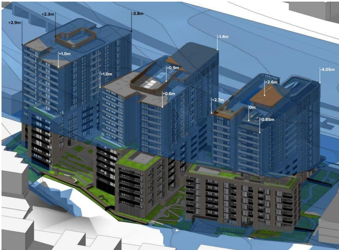
**Figure 32 |** Modelling showing areas of building height non-compliance with the blue plane representing the 48m building height limit (Source: Applicant’s RTS)
