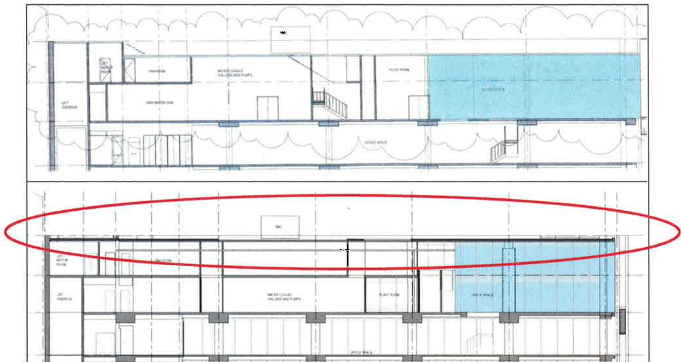
Figure 4: Approved (top) and proposed (bottom) section through roof levels, indicating the proposed increase of 400mm in roof height (source: Proponent (MOD 4 and MOD 5))
