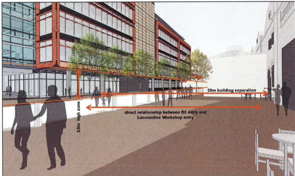
Figure 29: Proposed setback and public domain treatment of Locomotive Street (Source: applicant's RTS)
