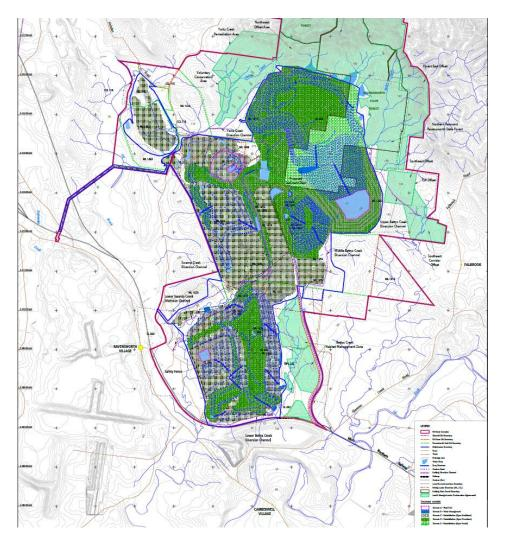
22 As such, it is evident that the current conceptual final landform design in the 2015 Approved MOP (as referred to in the approved LMP) provides for three final voids across the Complex, including a final void at Ravensworth East.
