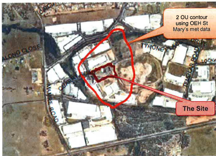
Figure 9: Maximum Hourly Tonnage - predicted ground level 2 OU concentrations, 99 th percentile, no air pollution control devices in operation (modelled as part of the RTS).
