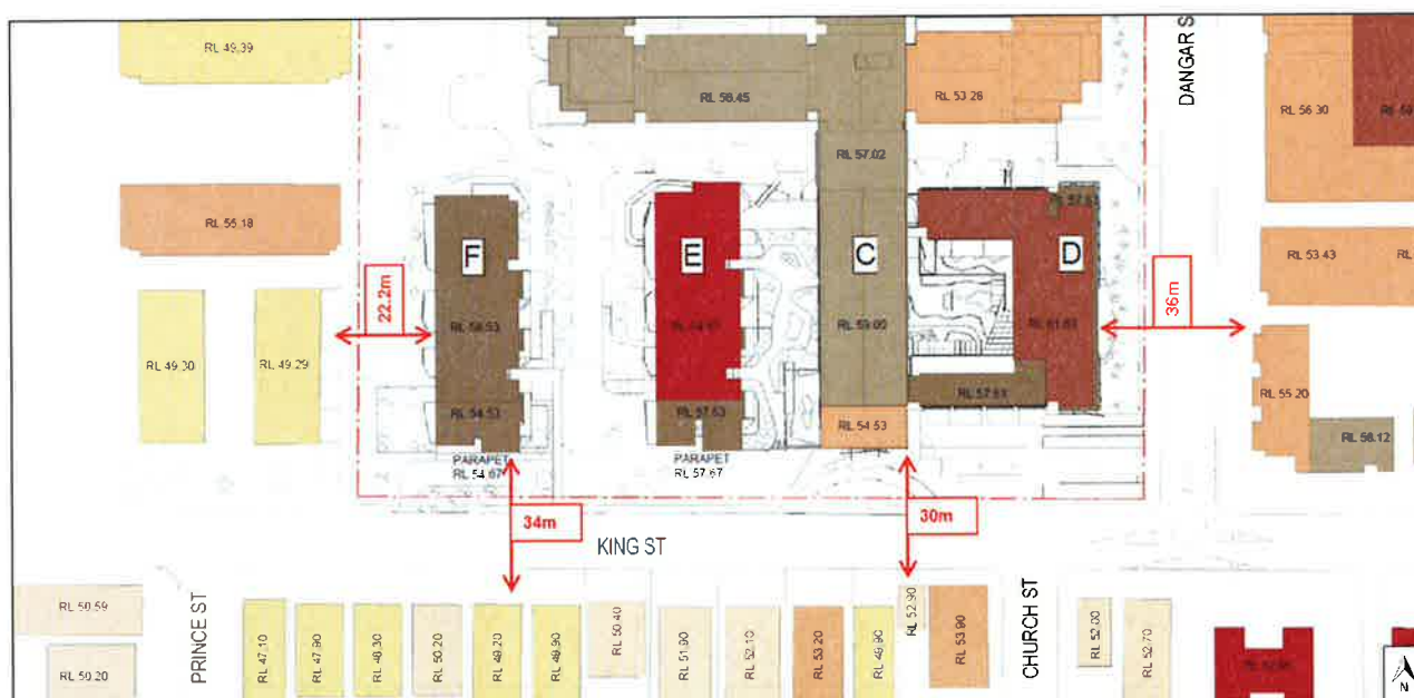
Figure 15: Building separation distances between the proposed building envelopes and neighbouring residential properties
