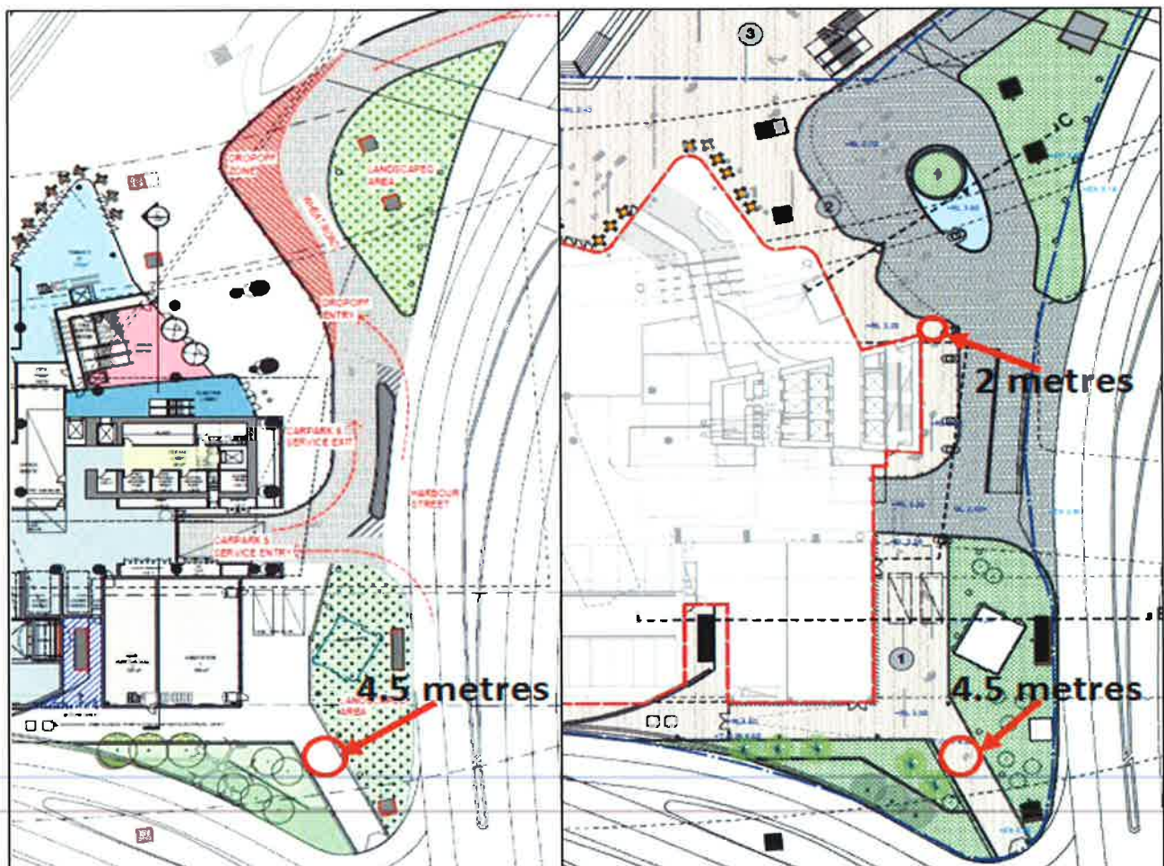
Figure 15: Comparison of the approved (left) and proposed (right) public domain upgrades to the east of the proposed building including approximate pedestrian pathway widths
