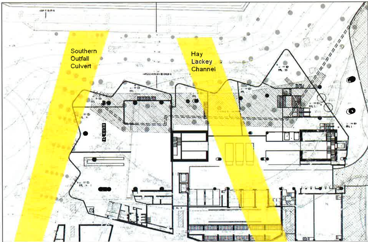
Figure 47: Approximate location of the Sydney Water stormwater assets (Base Image Source: Applicant's EIS)
